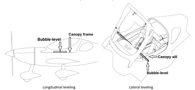
Fig. 6-1 Aircraft leveling
