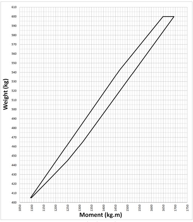
Fig. 6-9 Operating weight and moment chart – Metric Units
