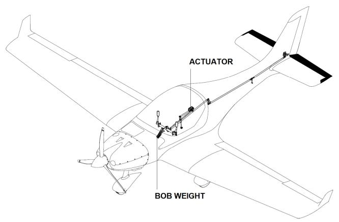
Fig. 7-2 *Elevator control*
