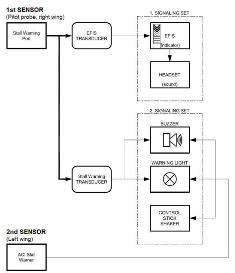
Fig. 7-32 Stall warning system schematic
