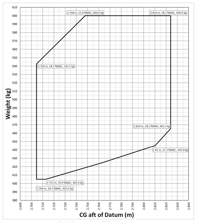
Fig. 6-2 Operating Weight /CG limit – Metric Units
