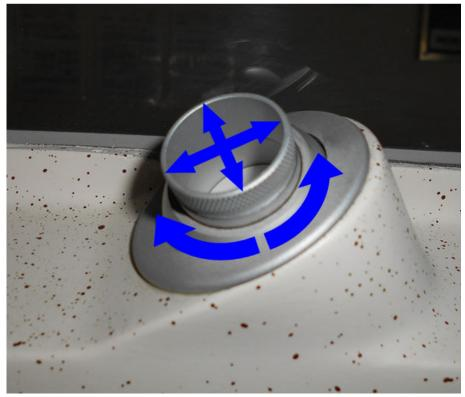
Fig. 7-29 Air outlets for cockpit venting
