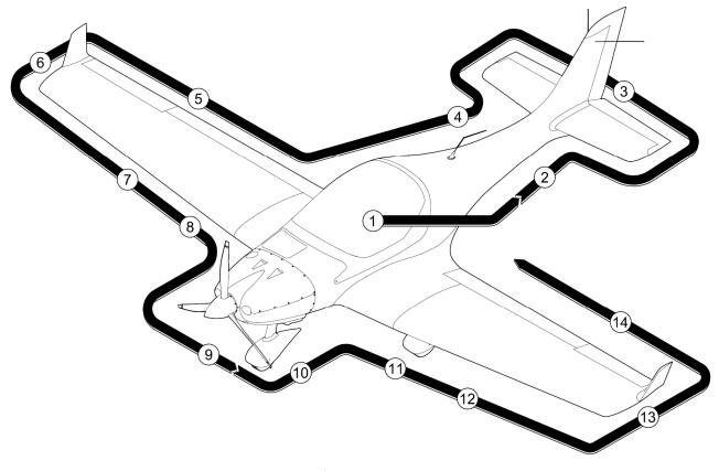
Fig. 4-1 Pre-flight inspection procedure
