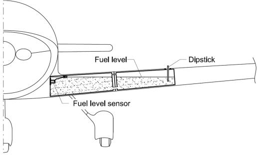
Fig. 7-26 Fuel quantity measurement
