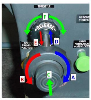
Fig. 7-15 Throttle controller
