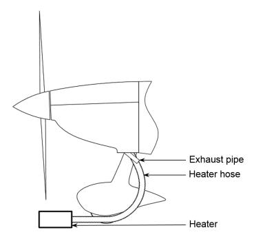
Fig. 8-6 Engine preheating
